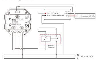
Note: We recommend the number of LED drivers connected to 0/1-10V dimmer does not exceed 100 pieces, The maximum length of the wires from dimmer to LED driver should be no more than 50 meters.
