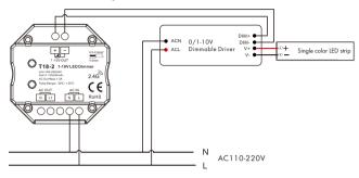
• Connect with 1-10V dimming driver (use AC OUT)
