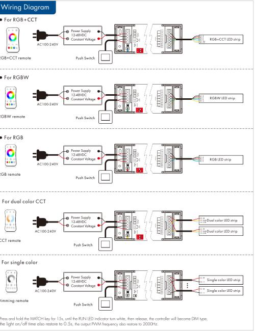
Note: 1. After changed the light type by DIP switch, please redo the tuya APP config operation. 2. For RGB+CCT or CCT light type, continuous power on and off will change 3 levels color temperature (WW, NW and CW) in sequence. 3. Switch off the power, then switch on power, repeat again. Immediately short press match key 3 times, the light on/off time will change between 3s and 0.5s.
