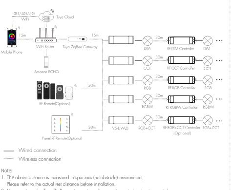
2. Users must use the Tuya ZigBee gateway to realize remote control and voice control.
