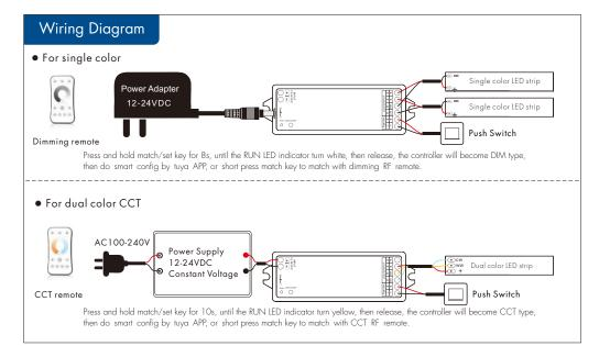
Note: 1. User can connect constant voltage power supply or power adapter as power input.
